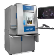
Bigfoot Spectral Sorter (6 lasers, 56 colours)
