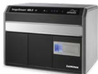
Amnis ImageStream X Mark II (3 lasers, 12 channels)
