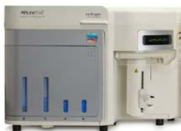
Attune NxT Flow Cytometer (3 lasers, 11 colours)
